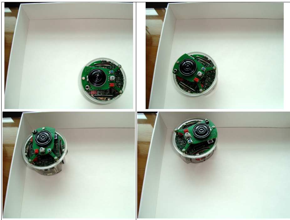
Fig. 6. Robot behavior in the real e-puck robot. The robot starts searching for a wall, when a wall is found, the epuck follows the wall while avoids crashing into walls.
