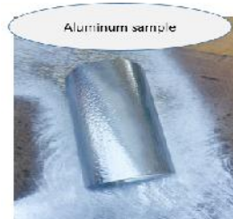
Figure 8: carbon steel pipe sample coated with aluminum.
