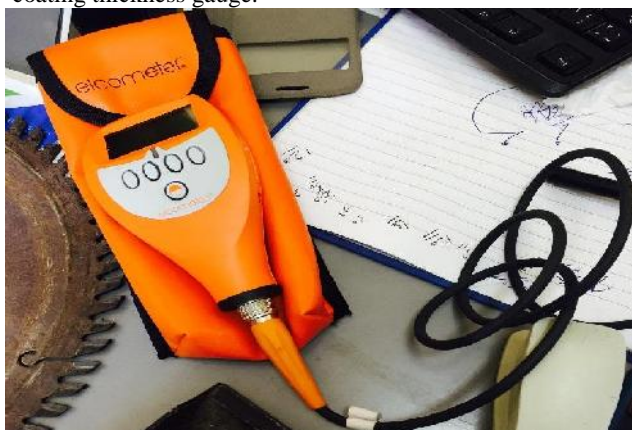
Figure 16: DFT (dry film thickness) device for measure thickness of coating.
